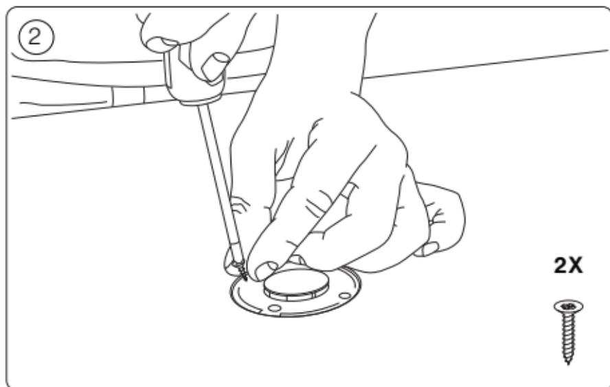
3. The screws activate the expansion mounting system.
